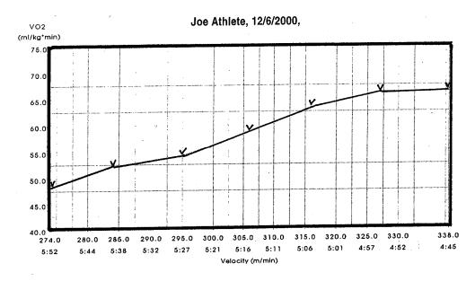
In Figure 2, the x-axis displays work in appropriate units of measurement and the y-axis displays  $VO_2$ , or oxygen uptake (ml/kg/min). Other variables are often recorded at each stage of the test. These include blood lactate, heart rate, and Rate of Perceived Exertion (not shown). Measurements obtained from the athlete during each stage of the test are plotted and displayed in this graphic format.
